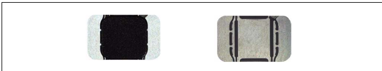
Figure 1-2 Pin configuration Module Contactless Card - MCC8 (top / bottom view)
