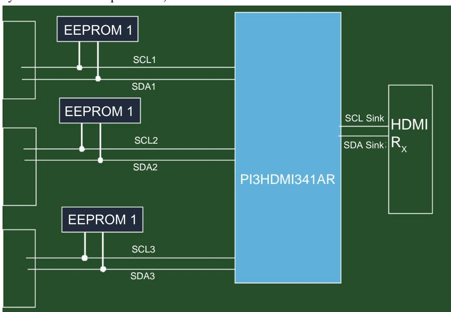
This architecture allows EDID readability when the DTV is power off or power on.
