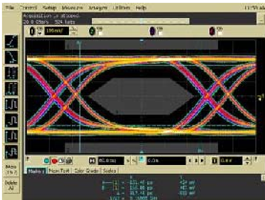
Figure 7: 12bit deep color DVI/HDMI TX eye tested with 1 meter. 30 AWG HDMI cable. Setting: Optimized equalization, 0dB output pre-emphasis and de-emphasis, and Swing 500mV.
