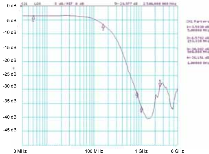
Figure 4 – Typical Insertion Loss Curve. Spikes at high frequencies are caused by PCB layout.
