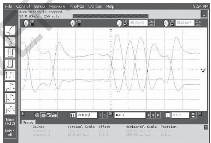
Data Waveforms, 2.5Gbps (left) & 5.0Gbps (right)
