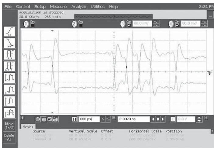
Data Waveforms, 2.5Gbps (left) & 5.0Gbps (right)
