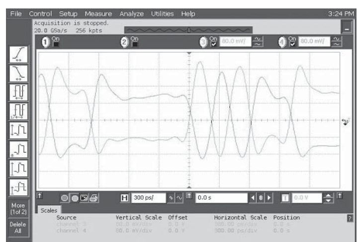
Data Waveforms, 2.5Gbps (left) & 5.0Gbps (right)
