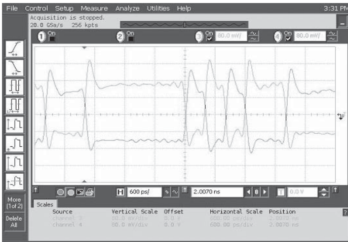
Data Waveforms, 2.5Gbps (left) & 5.0Gbps (right)
