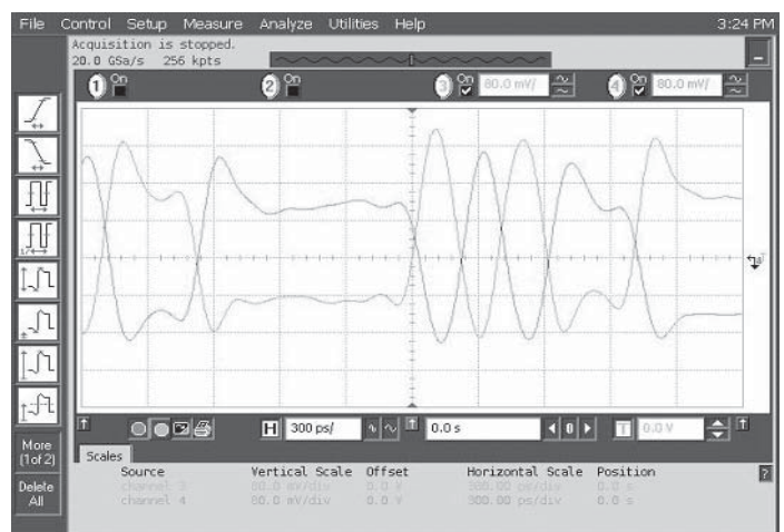
Data Waveforms, 2.5Gbps (left) & 5.0Gbps (right)
