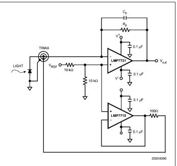
FIGURE 3. LMP7721 as Transimpedance Amplifier
