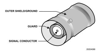
FIGURE 1. The Structure of a Triax
