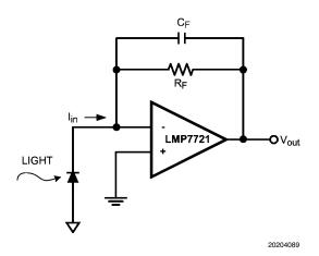
FIGURE 2. Photodiode Transimpedance Amplifier
