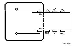
FIGURE 6. Circuit Board Guard Layout
