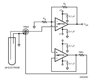
FIGURE 5. LMP7721 as pH Electrode Amplifier
