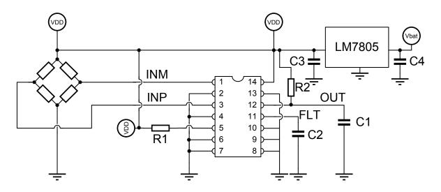
With the use of an external voltage regulator to supply the sensor, the MLX90326 as well as an ADC used for converting the analog output signal, the MLX90326 can be used in a non ratio-metric mode. An example of standard voltage regulator is the LM7805. C1, C2, R1 and R2 are the same as in the ratio-metric application mode. C4 has a typical value of 330nF and C3 of 100nF in this application mode.
