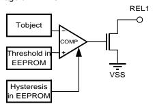
The comparator is a digital comparator, with a resolution of 12 bits. By default the input polarity is inverting. Threshold and hyteresis values are version dependent, as indicated below. These settings can be changed by factory programming on request.
