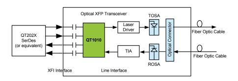
System Block Diagram with the QT1010
