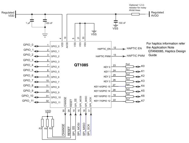
Pin 33 is the pad on the underside of the device which should be connected to Vss.
