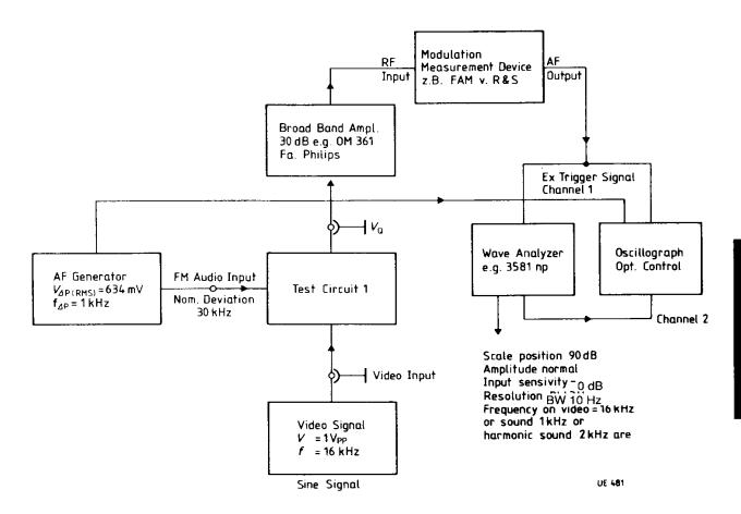
Calibration: AF signals are switched off, video signal is present at video input, modulation measurement device set at AM is adjusted to video carrier; filter: 300 Hz ... 20 kHz; detector: (P + P)/2; wave analyzer at video signal level (16 kHz) adjusted and resultant level as reference av defined.
