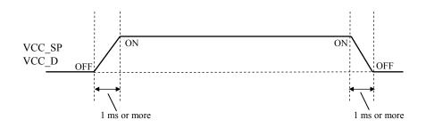
Note) \*1 : This IC contains the pre-charge circuit, It is time until each bias is stabilized from Standby OFF.
