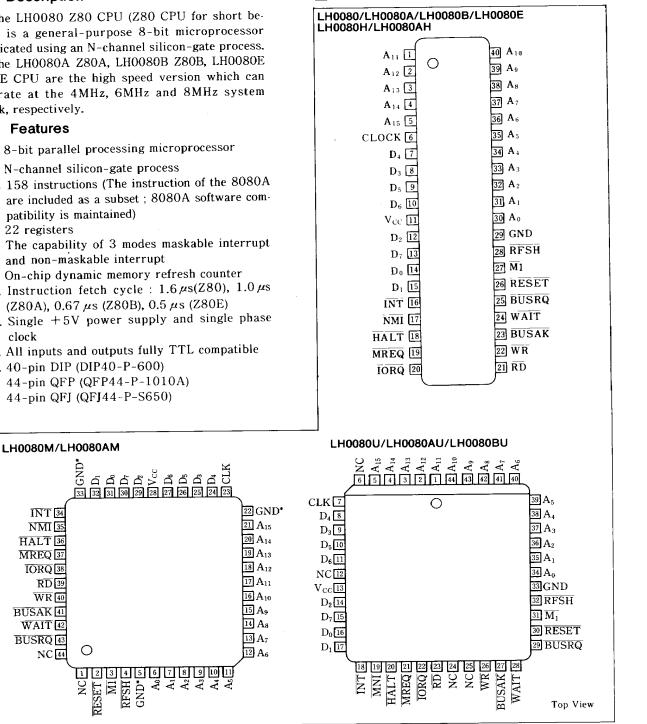
\* The GND pins must be connected to the GND level.
