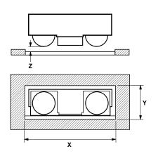
X is the width of the window, Y is the height of the window, and Z is the distance from the HSDL-3202 to the back of the window. The distance from the center of the LED lens to the center of the photodiode lens is 5.1 mm. The equations for the size of the window are as follows:
