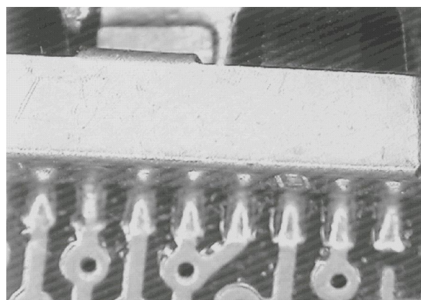
Photo 4.0. Unit self-aligns after reflow.
