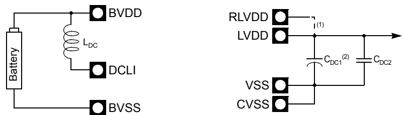
Figure 135. Battery DC-DC Connection
