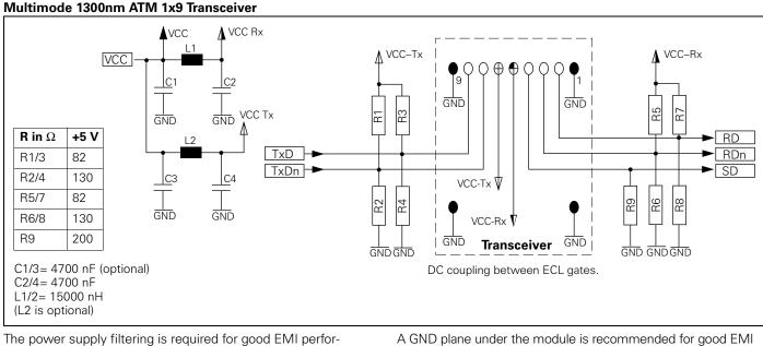
The power supply filtering is required for good EMI performance. Use short tracks from the inductor L1/L2 to the module  $V_{CC}$ -Rx/ $V_{CC}$ -Tx.
