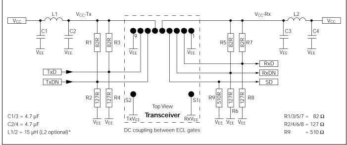
$<sup>^*</sup>$  Recommended choke is Siemens Matsushita B78108-S1153-K or B78148-S1153-K ( $Q_{min}$ =60, max. DC resistance=0.6  $\Omega$ )
