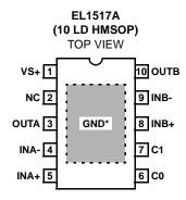
THERMAL PAD MUST BE CONNECTED TO GROUND. PAD IS CONNECTED INTERNALLY TO  $V_{S^-}$  AND THUS EL1517A CAN ONLY BE USED IN SINGLE SUPPLY APPLICATIONS.
