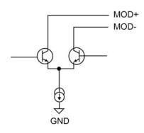
Figure 1c. Simplified Driver Output Stage
