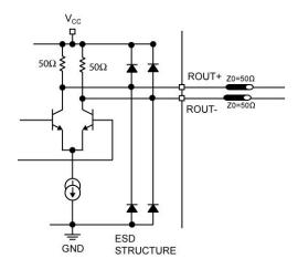
Figure 1e. Post Amplifier Output Stage
