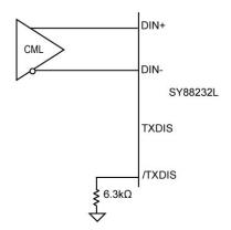
Figure 2b. Driving DIN with CML Outputs<sup>(1)</sup>
