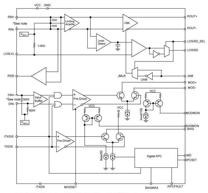
\*note: The internal terminations at DIN+, DIN-, RIN+, RIN- apply for SY88232L only. SY88232AL doesn't have internal terminations at those inputs
