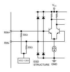
Figure 1d. Post Amplifier Input Stage<sup>(1)</sup>
