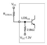
Figure 2c. LOSLVL Setting Circuit
