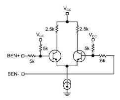
Figure 1b. Simplified TXDIS Input Stage
