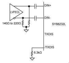
Figure 2a. Driving DIN with PECL Outputs<sup>(1)</sup>
