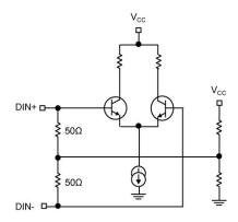
Figure 1a. Simplified Driver Input  ${\rm Stage}^{(1)}$
