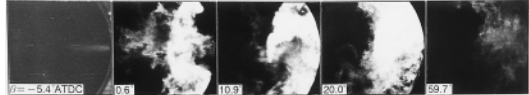
ATDC: After Top Dead Center, \theta : Crank angle with respect to ATDC How soot is generated can be observed by viewing low-level scattering light resulting from laser irradiation.
