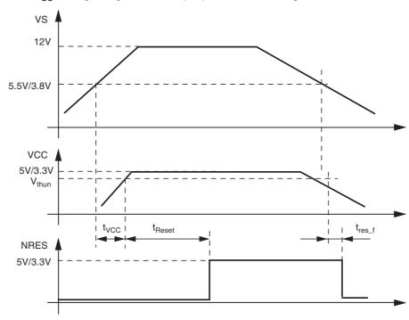
**Figure 6-1.** V<sub>CC</sub> Voltage Regulator: Ramp Up and Undervoltage
