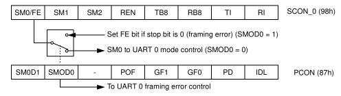
Figure 21. UART 1 Framing Error Block Diagram
