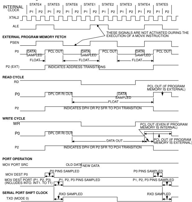
This diagram indicates when signals are clocked internally. The time it takes the signals to propagate to the pins, however, ranges from 25 to 125 ns. This propagation delay is dependent on variables such as temperature and pin loading. Propagation also varies from output to output and component. Typically though ( $T_A = 25$ °C fully loaded)  $\overline{RD}$  and  $\overline{RD}$  and  $\overline{RD}$  and  $\overline{RD}$  and  $\overline{RD}$  are incorporated in the AC specifications.
