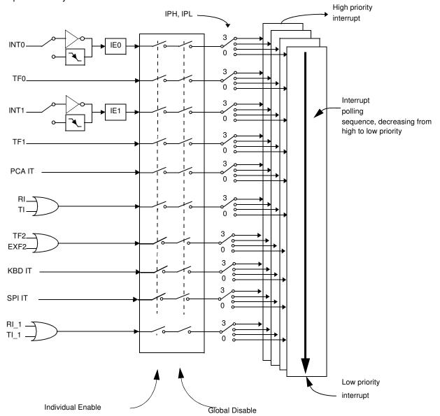
Each of the interrupt sources can be individually enabled or disabled by setting or clearing a bit in the Interrupt Enable register (Table 78 and Table 76). This register also contains a global disable bit, which must be cleared to disable all interrupts at once.
