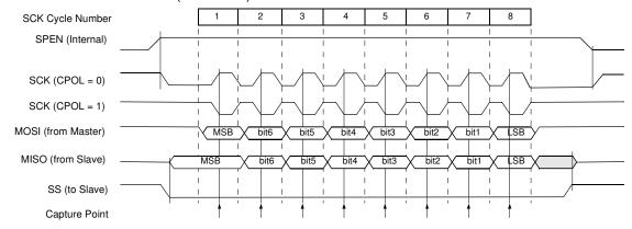
Figure 37. Data Transmission Format (CPHA = 1)
