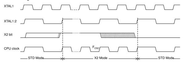
The X2 bit in the CKCON0 register (see Table 14) allows a switch from 12 clock periods per instruction to 6 clock periods and vice versa. At reset, the speed is set according to X2 bit of the Fuse Configuration Byte (FCB). By default, Standard mode is active. Setting the X2 bit activates the X2 feature (X2 mode).
