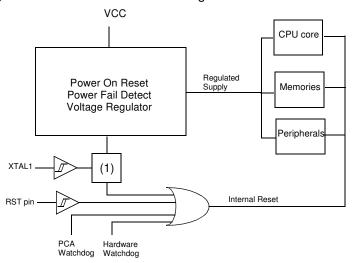
Note: 1. Once XTAL1 High and low levels reach above and below VIH/VIL. a 1024 clock period delay will extend the reset coming from the Power Fail Detect. If the power falls below the Power Fail Detect threshold level, the Reset will be applied immediately.
