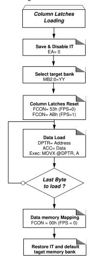
Note: The last page address used when loading the column latch is the one used to select the page programming address.
