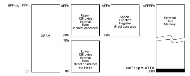
When an instruction accesses an internal location above address 7Fh, the CPU knows whether the access is to the upper 128 bytes of data RAM or to SFR space by the addressing mode used in the instruction.
