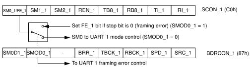
When this feature is enabled, the receiver checks each incoming data frame for a valid stop bit. An invalid stop bit may result from noise on the serial lines or from simultaneous transmission by two CPUs. If a valid stop bit is not found, the Framing Error bit (FE) in SCON register (See Table 62.) bit is set.
