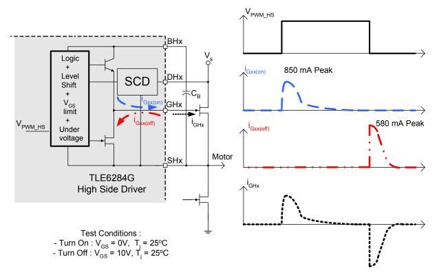
This figure represents the simplified internal circuit of one high side gate drive. The drive circuit of the low sides look similar.
