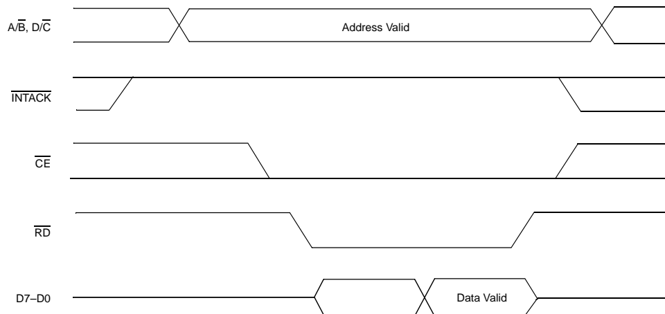
Figure 21. Read Cycle Timing
