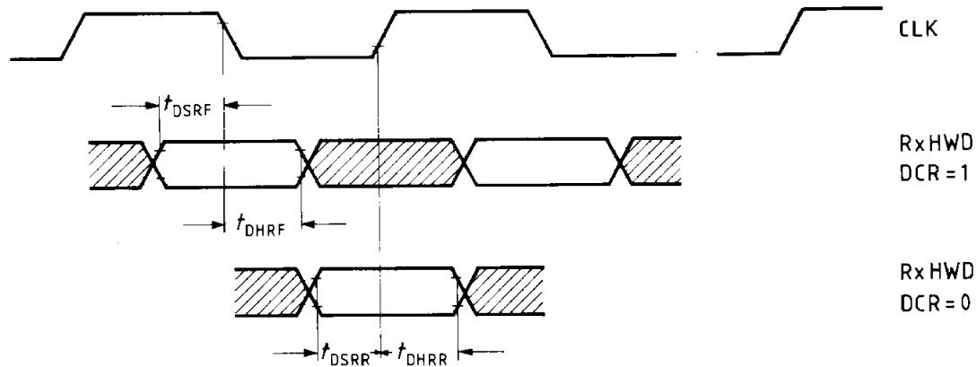
\*) Common channel mode  $t_{DSRR}$  75 ns
