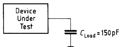
AC testing: inputs are driven at 2.4 V for a logic "1" and at 0.45 V for a logic "0".
