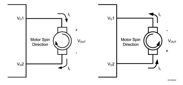
FIGURE 2. Voltage Polarity and Motor Direction
