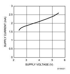
Shutdown Supply Current vs Supply Voltage
