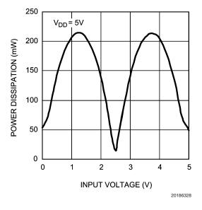
FIGURE 3. Power Dissipation vs. Input Voltage
