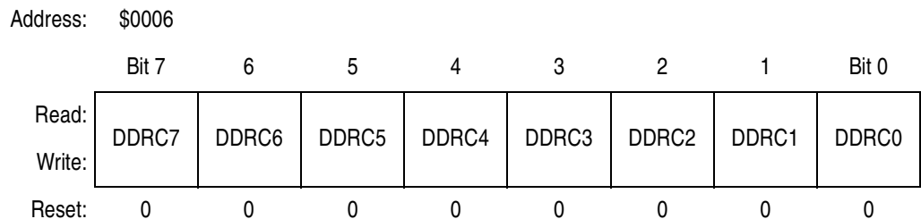
Figure 7-8. Data Direction Register C (DDRC)
