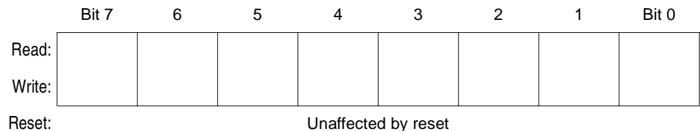
Figure 3-3. Index Register (X)
