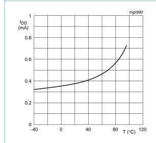
$V_{DD} = 3 \text{ V}$ ; Timer = 1 minute.
