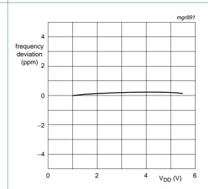
$T_{amb}$  = 25 °C; normalized to  $V_{DD}$  = 3 V.
