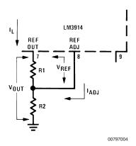
Since the  $120\mu A$  current (max) from the adjust terminal represents an error term, the reference was designed to minimize changes of this current with V<sup>+</sup> and load changes.
