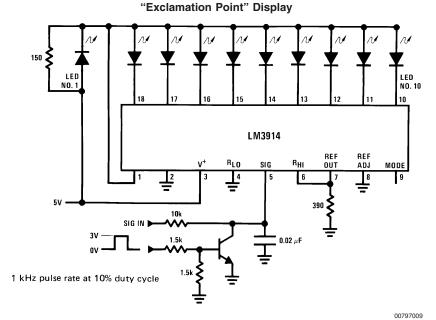
LEDs light up as illustrated with the upper lit LED indicating the actual input voltage. The display appears to increase resolution and provides an analog indication of overrange.
