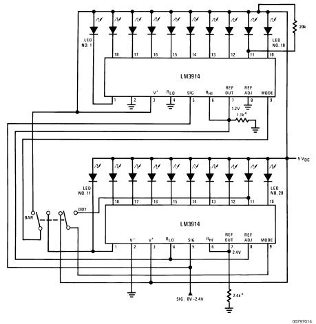
\*The exact wiring arrangement of this schematic shows the need for Mode Select (pin 9) to sense the V<sup>+</sup> voltage exactly as it appears on pin 3. Programs LEDs to 10mA
