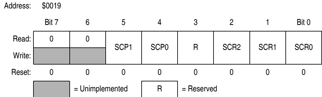
Figure 16-18. SCI Baud Rate Register (SCBR)
