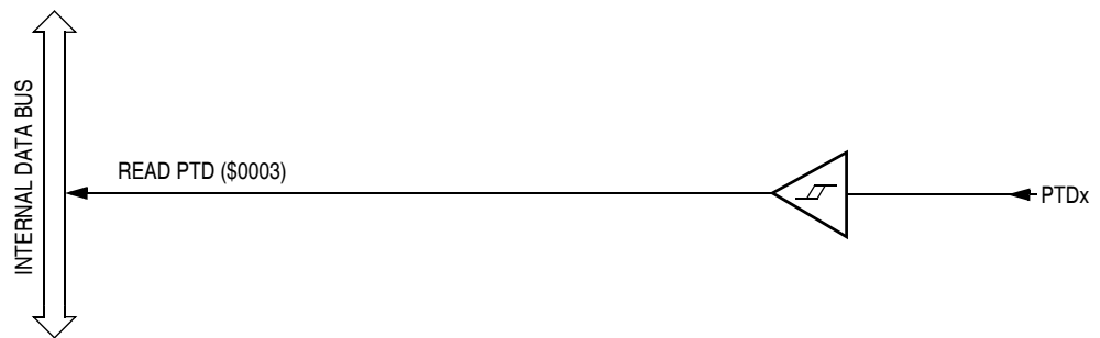
Figure 15-12. Port D Input Circuit
