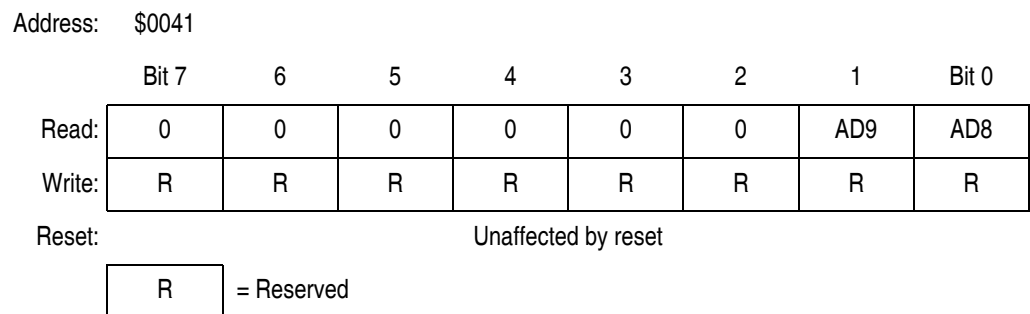
Figure 19-5. ADC Data Register High (ADRH) Right Justified Mode
