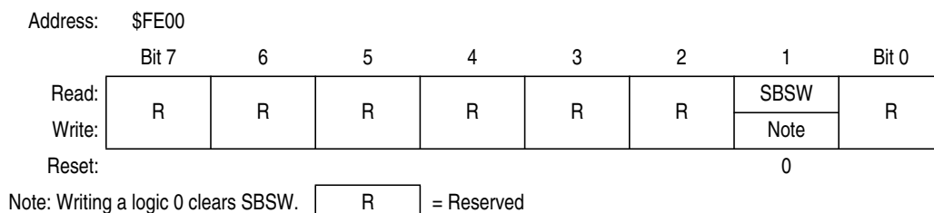
Figure 21-6. SIM Break Status Register (SBSR)
