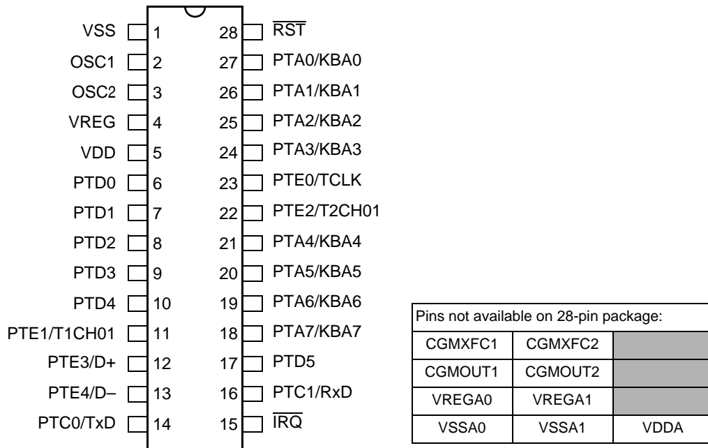
Figure 1-3. 28-Pin SOIC Pin Assignment
