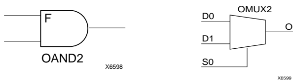
Figure 20: AND & MUX Symbols in XC4000X IOB
