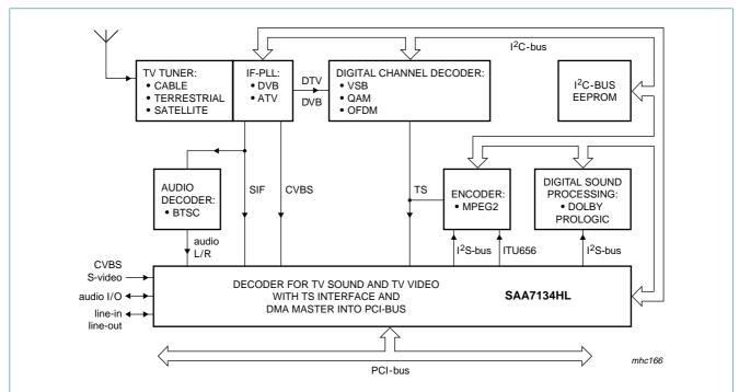
Fig 1. Application diagram for capturing live TV video and audio streams in the PC, with optional extensions for enhanced audio feature processing or DTV and DVB capture
