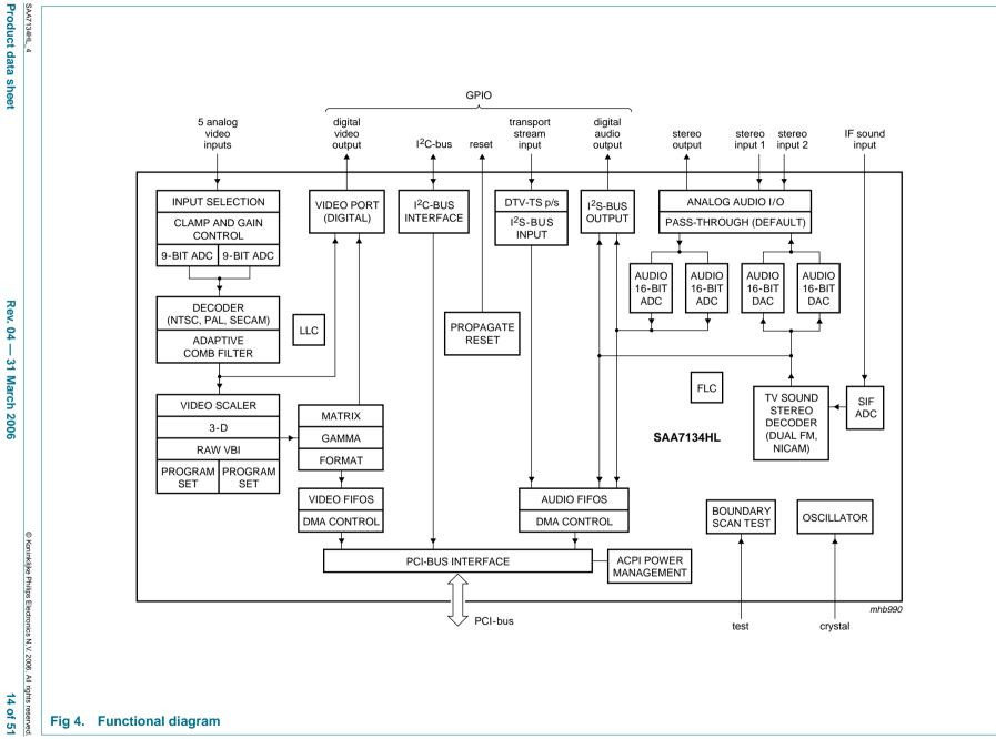
Audio, video and transport streams are collected in a configurable FIFO with a total capacity of 1 kB. The DMA controller monitors the FIFO filling degree and master-writes the audio and video stream to the associated DMA channel. The virtual memory address space (from OS) is translated into physical (bus) addresses by the on-chip hardware Memory Management Unit (MMU).
