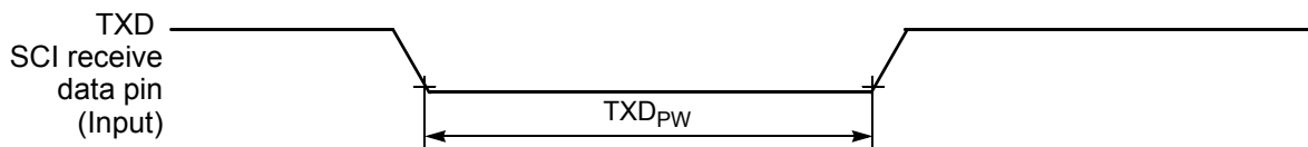
Figure 10-17 TXD Pulse Width
