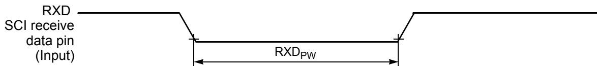
Figure 10-16 RXD Pulse Width
