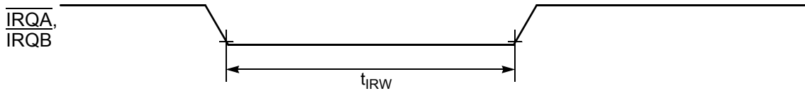
Figure 10-6 External Interrupt Timing (Negative-Edge Sensitive)
