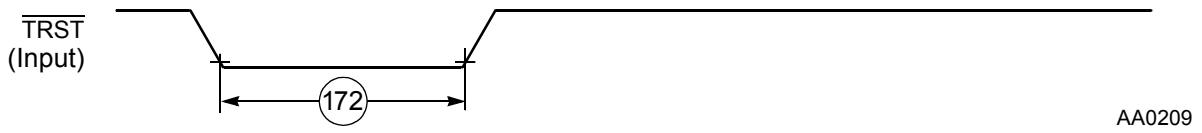
Figure 36. \overline{\text{TRST}} Timing Diagram
