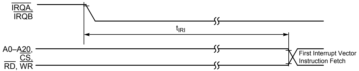
Figure 4-14 Interrupt from Wait State Timing
