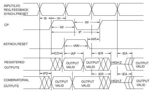
Note: 1. Timing measurement reference is 1.5V. Input AC driving levels are 0.0V and 3.0V, unless otherwise specified. **AC Characteristics for the ATV2500L**
