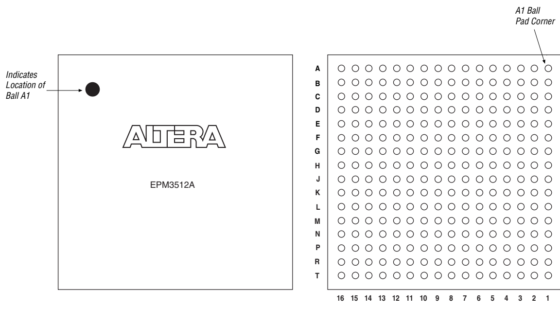
Figure 18. 256-Pin FineLine BGA Package Pin-Out Diagram
