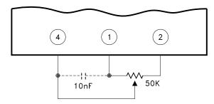
Adjust/comp (pin 4) may be driven by external circuitry referenced to pin 2 (-output) if desired. Grounding pin 4 causes voltage to increase (25% typically) while driving pin 4 above 1.3V causes output voltage to decrease. Pin 4 may be driven negative without damage, however the resultant increase in converter output voltage should be considered. Pin 4 may be driven through  $10 \mathrm{K}\Omega$  or more if connection of the comp function is also required.
