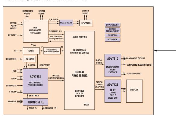
The ADV7402 and ADV7400 multiformat video decoders simplify front end digitizer and decoder architectures by reducing board space, simplifying auto detection and switching of inputs, and reducing overall system power consumption.
