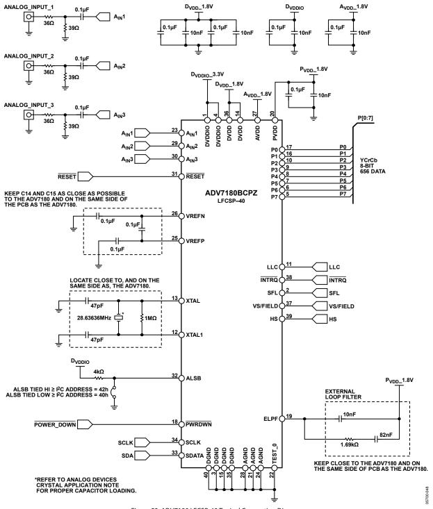
Figure 53. ADV7180 LFCSP-40 Typical Connection Diagram
