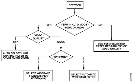
Figure 18. YSFM and WYSFM Control Flowchart
