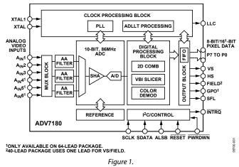
sources. AGC and clamp-restore circuitry allow an input video signal peak-to-peak range up to 1.0 V. Alternatively, these can be bypassed for manual settings.
