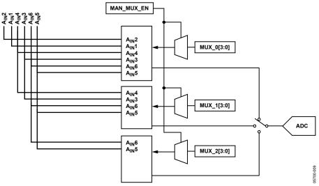
Figure 9. Internal Pin Connections LQFP-64
