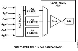
Figure 12. Antialias Filter Configuration
