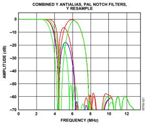
Figure 21. Y S-VHS 18 Extra Wideband Filter (CCIR 601 Compliant)
