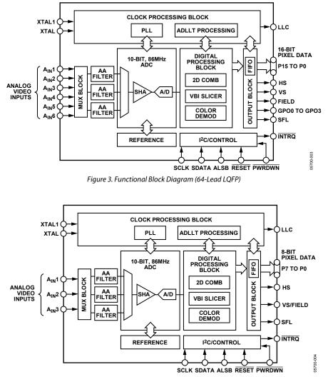
Figure 4. Functional Block Diagram (40-Lead LFCSP)
