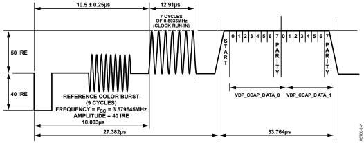
Figure 45. CCAP Waveform and Decoded Data Correlation
