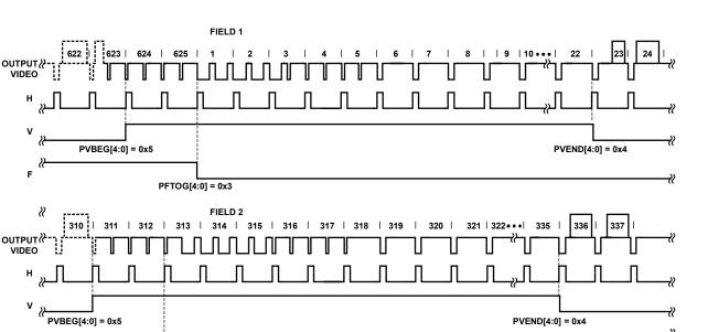
Figure 38. PAL Default, ITU-R BT.656 (the Polarity of H, V, and F is Embedded in the Data)
