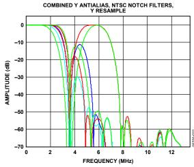
Figure 22. Y S-VHS 18 Extra Wideband Filter (CCIR 601 Compliant)
