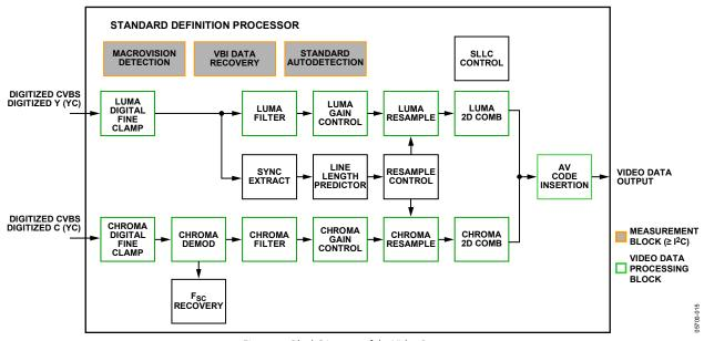
Figure 15. Block Diagram of the Video Processor
