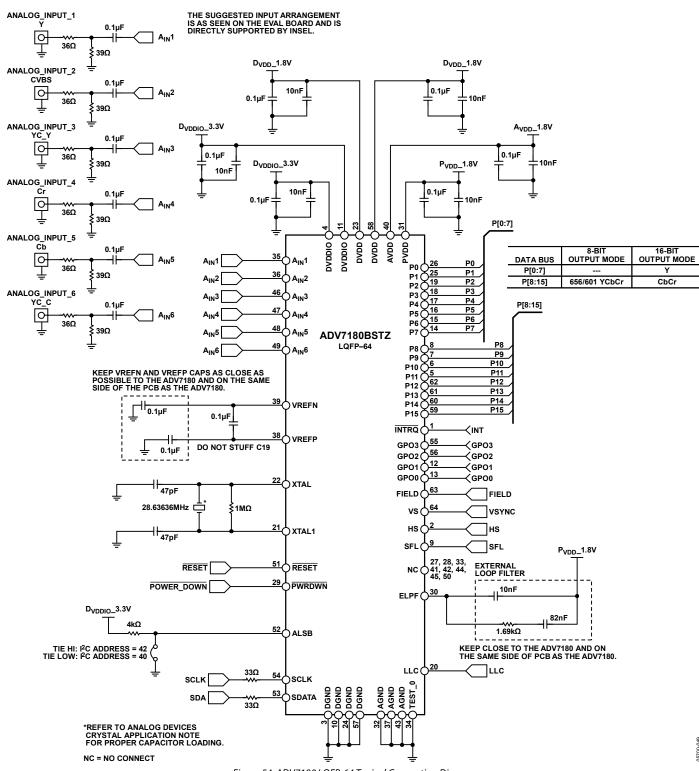
Figure 54. ADV7180 LQFP-64 Typical Connection Diagram
