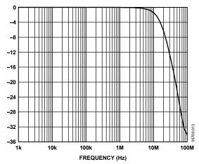
Figure 13. Antialiasing Filter Magnitude Response
