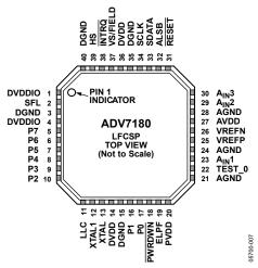
Figure 7. 40-Lead LFCSP Pin Configuration
