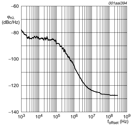
Fig 8. Phase noise density as function of offset frequency (low band); typical values
