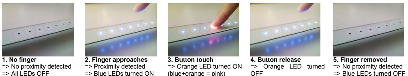
Figure 66 Touch+Proximity Module Operation
