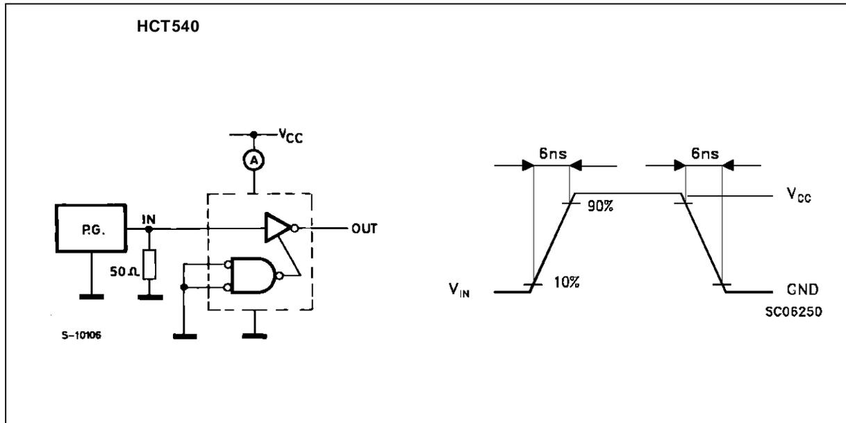
SWITCHING CHARACTERISTICS TEST CIRCUIT
