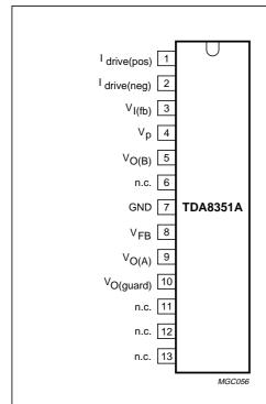
The die has been glued to the metal block of the package. If the metal block is not insulated from the heat sink, the heat sink may only be connected directly to pin 7.
